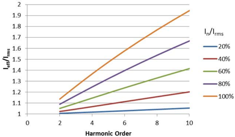
Figure 8-2 Ratio of effective conductor current to the actual rms current for fundamental current plus various levels of single-frequency harmonic distortion, as a function of the harmonic order of the distortion, for a 2167 kcmil ACSR (Kiwi) conductor.
